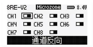
Using Channel 1 as an example, when the blackened rectangle icon is on the left, toggling the rocker from left to right will cause the servo to swing from left to right (Fig. 1), and when the blackened rectangle icon is on the right, toggling the rocker from left to right will cause the servo to swing from right to left (Fig. 2).
