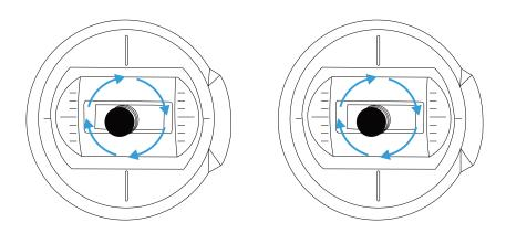
Then pull the rocker to the center position as shown below, and finally pull the D/R switch, the calibration is complete.
