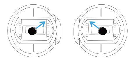
At the same time, turn on the power of the remote control and enter into the joystick calibration state, first pull the two joysticks of the remote control left, right, up, down and to the maximum extent as shown in the figure below,
